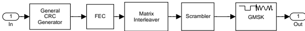
Figure 12. Illustration of blocks in implementation of the Mobitex protocol in the transmitter
