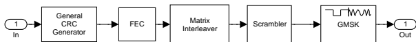
Figure 12. Illustration of blocks in implementation of the Mobitex protocol in the transmitter
